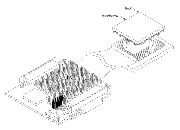
Figure 1–3: Placing the microprocessor into the probe adapter
