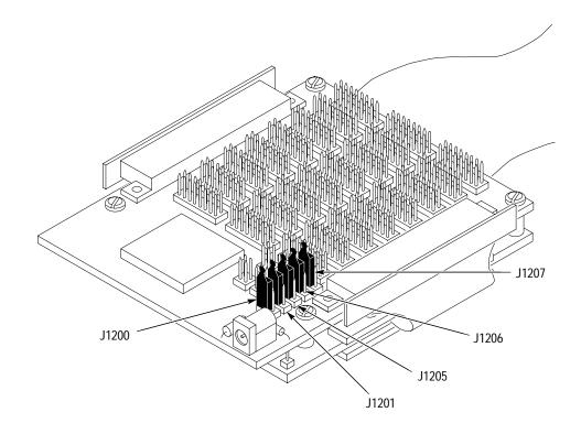
Figure 1–1: Jumper locations on the probe adapter
