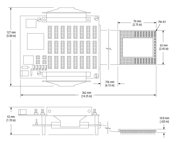
Figure 3–3: Dimensions of the probe adapter
