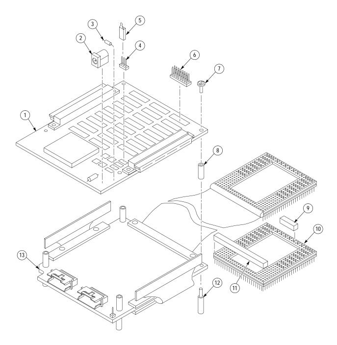
Figure 1: Pentium Pro probe adapter exploded view
