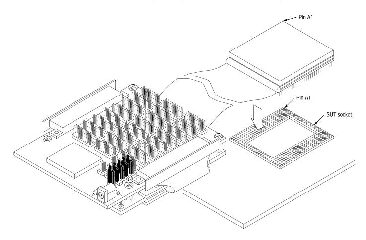
Figure 1-4: Placing the probe adapter onto the SUT
