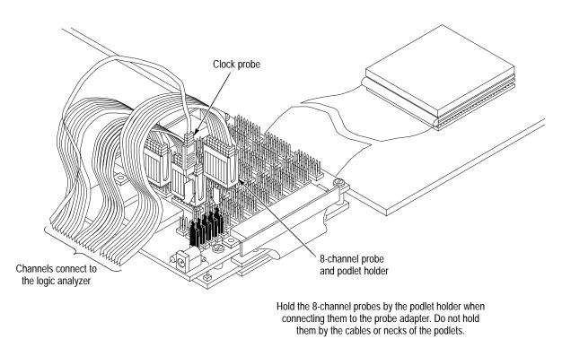
Figure 1–5: Connecting the probes to the probe adapter
