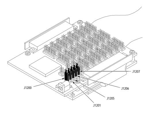
Figure 3–1: Jumper locations on the probe adapter
